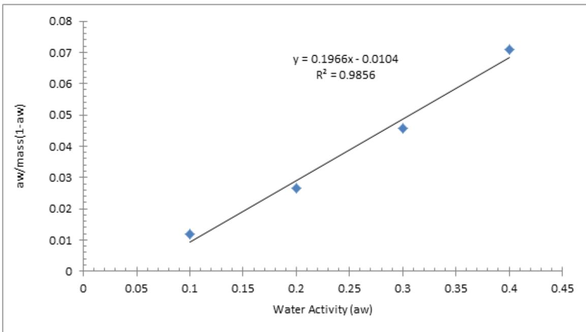
Figure 7: BET plot of wheat-yam (75:25) noodles at 32 and 37°C
